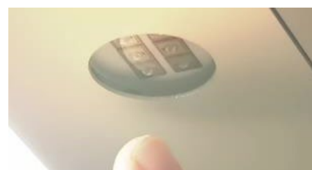
Illustration 5600 mW UVC-LED module in the Binz RESCUBE 3 (Fraunhofer IOSB-AST / Binz automotive)
