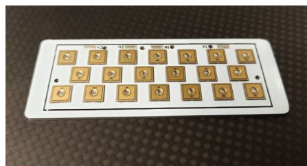
Illustration 3 2.1 Watt UVC-LED module 265 nm (Fraunhofer IOSB-AST)
